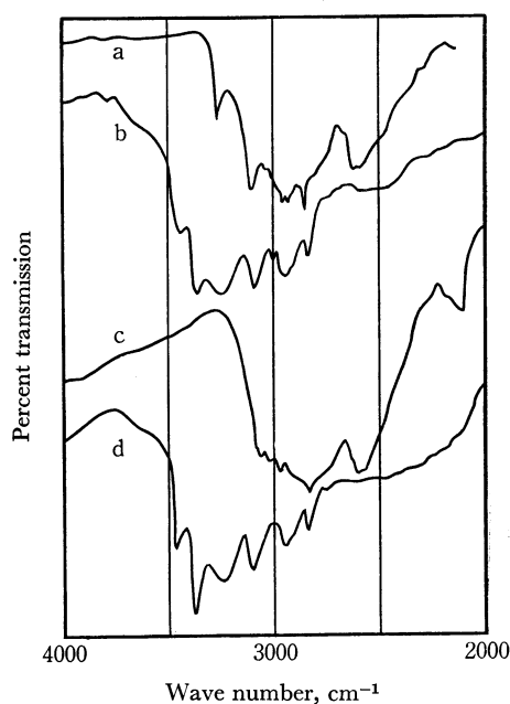
Fig. 1. Vibrational spectra, a) the p -anisidine-2,4-dinitrophenol at room temperature, b) the same above the melting point, c) the m -anisidine-2,4-dinitrophenol at room temperature, and d) the same above the melting point.
